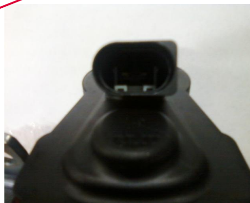
DC784634E (left) DC784635E (right) Plain connector Calipers fitted prior to 2008
