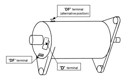
Do not over tension the fan belt, a dynamo belt does not require the same tension as an alternator belt. Over tightening the belt will cause the rear bush to fail.
